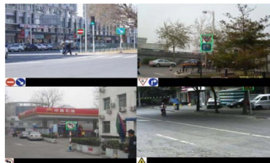
Fig.19 Some experimental results of traffic sign detection and recognition in complex urban scenes
